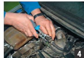
To couple fuel lines, clamps of plastic materials are used; with metal clamps, a spark might go off.
