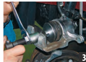
By rotating the handle or by using a socket wrench, push the brake piston into the starting position.
