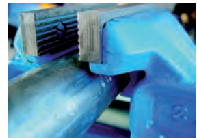
The lower end of the jaw is designed for clamping of tubes.
