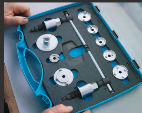
A suitable adapter that accurately fits the size of the brake piston must be selected.
