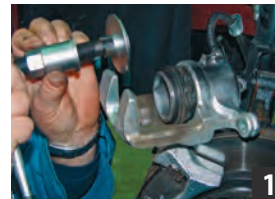
Mount the body of the tools with the suitable thread for compressing the pistons on the caliper.
