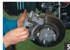
Remove the disc spreader and mount the brake caliper on the mounting boss.
