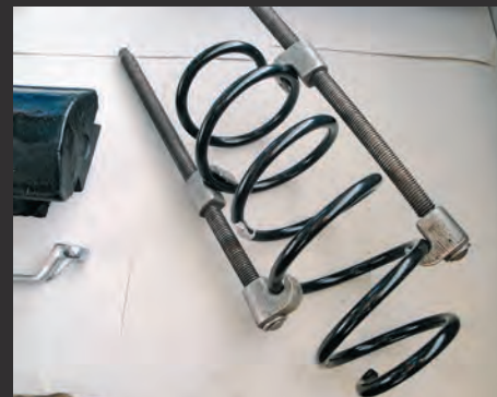
The older version of a simple tool for removing shock absorbers, which is not reliable enough.
