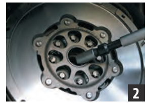
The socket size should suit the flywheel.
