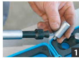
Choose a socket of a suitable size.
